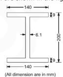
The plastic section modulus about the weaker axis (in  $cm^3$ , up to one decimal place) is \_\_\_\_\_
