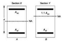
Due to presence of more compression steel in section Y, NA of section of Y is above than as of X. It means Y is more under-
