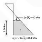
Earth pressure when tension cracks are developed
