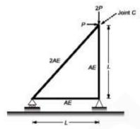
Given that  $E = 2 \times 10^{11} \, \text{N/m}^2$ ,  $A = 10 \, \text{mm}^2$ ,  $L = 1 \, \text{m}$  and  $P = 1 \, \text{kN}$ . the horizontal displacement of Joint C (in mm, up to one decimal place) is \_\_\_\_\_.
