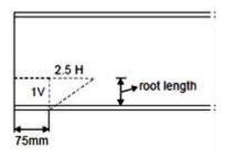
Effective area in bearing =  $[75 + 2.5 \text{ (flange thickness + root radius)}] \times 8$
