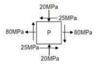
By how much angle  $(\theta)$  in degrees the stress element should be rotated in order to get the planes of maximum shear stress?
