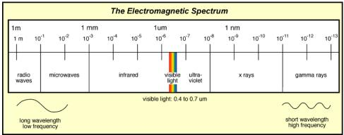
Infrared radiation, what we experience as heat when we hold our hand near a warm object, is somewhat longer wavelengths than visible light. Visible light is simply electromagnetic radiation in a range of wavelengths that our eyes are sensitive to. Visible wavelengths range from 0.0007 milimeters for red light, through orange, yellow, green, and blue, to 0.0004 milimeters for violet light. Ultraviolet is shorter wavelengths than violet.
