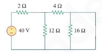
The current through the short-circuited path or 4 ohm resistor is
