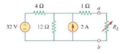
For calculating thevenin's resistance, all the source are replaced by their internal resistances.
