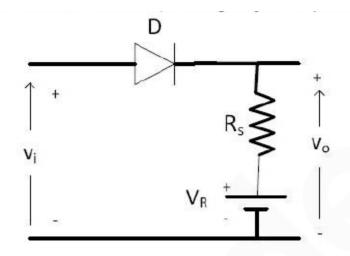
For the positive half cycle, the diode is forward biased when the input voltage is greater than  $V_{\rm \tiny R}$
