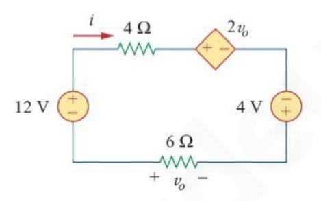
Applying KVL analysis in the loop
