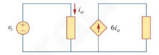
The dependent source given in the circuit is current controlled current source.
