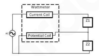
The wattmeter reads the power consumed by the load  $Z_2$  because the potential coil is placed in parallel to the load and current coil will have the current through it.
