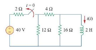
For t < 0 the inductor will behave as short-circuited and hence the circuit reduces to
