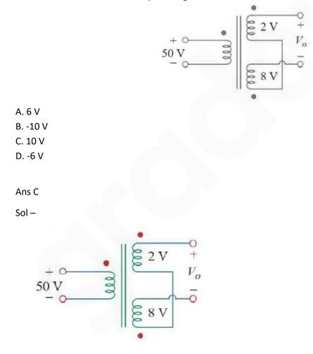
Let the current entering to the winding at dot side be positive terminal
