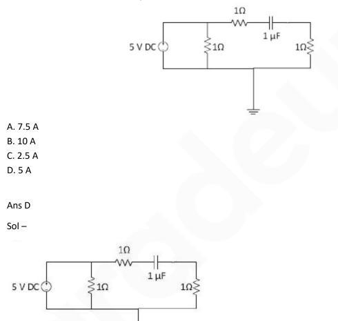
At steady state, the capacitor will behave as open-circuited.
