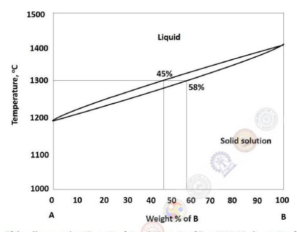
If the alloy contains 47 wt. % of A and 53 wt. % of B at 1300 °C, the wt. % of liquid present in the alloy at this temperature will be .......
