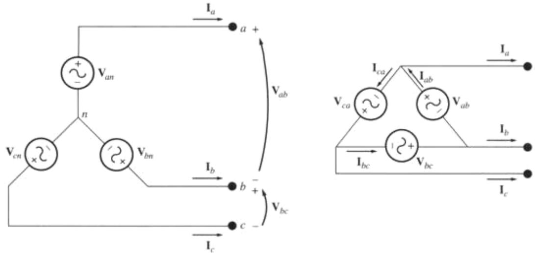
Each generator and each load can be either **Y**- or  **$\Delta$** -connected. Any number of **Y**- and  **$\Delta$** -connected elements may be mixed in a power system.
