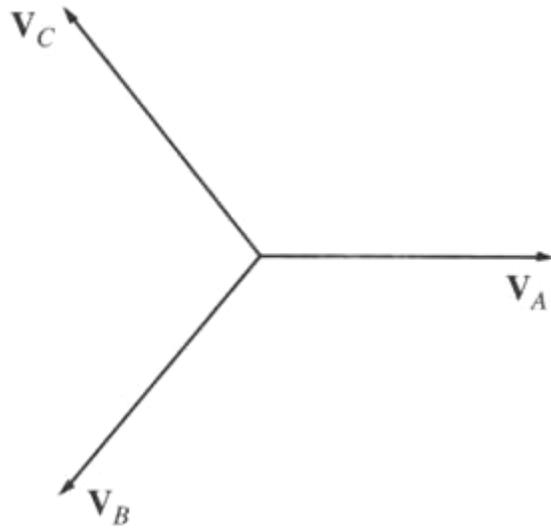
$$I_A = \frac{V \angle 0^\circ}{Z \angle \theta} = I \angle -\theta$$
