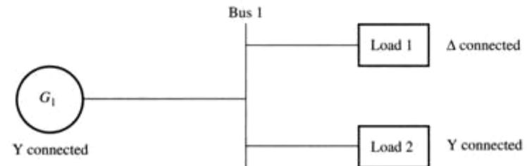
If we can neglect the impedance of the transmission line, an important simplification in the power calculation is possible...
