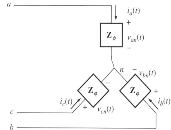
$$p_a(t) = v_{an}(t)i_a(t) = 2VI \sin(\omega t) \sin(\omega t - \theta)$$
