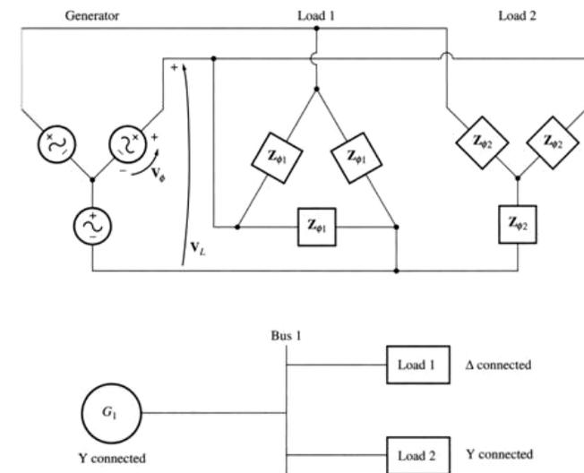
We can treat the line voltage as constant and use the power triangle method to quickly calculate the effect of adding a load on the overall system and power factor.
