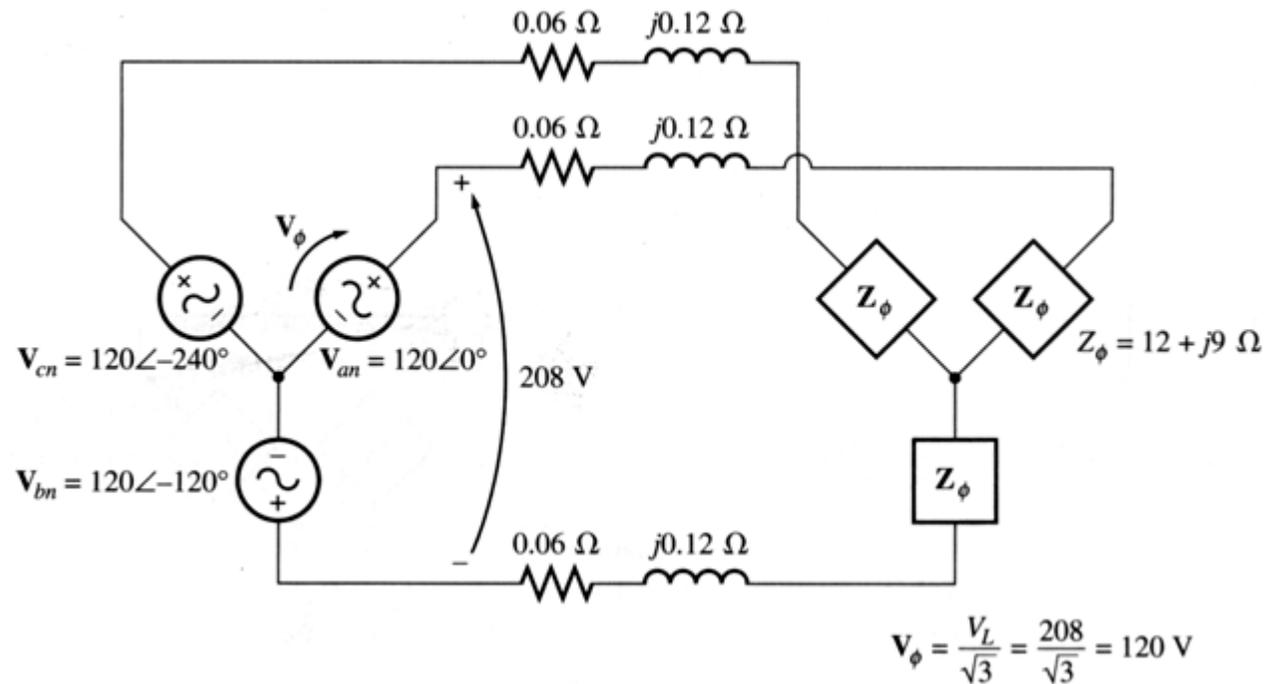
Both, the generator and the load are Y-connected, therefore, it's easy to construct a per-phase equivalent circuit.
