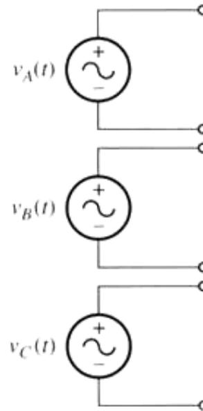
$$v_A(t) = \sqrt{2} V \sin \omega t \text{ V}$$
