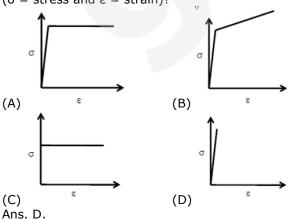
A **stress-strain** curve is a graph derived from measuring load (stress -  $\sigma$ ) versus extension (strain -  $\epsilon$ ) for a sample of a material. The nature of the curve varies from material to material.
