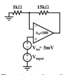
The output voltage (in millivolts) is \_\_\_\_\_
