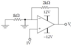
A. 10 Volts B. 12.5 Volts C. 12 Volts D. 15 Volts Answer | | | C Solution | | | Correct answer is 12. For the given op-amp,  $V_+ > V_-$ So,  $V_{out} = V_{saturation} = 12 \text{ Volts}$
