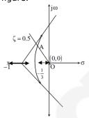
The constant damping ratio line, for  $\xi=0.5$ , intersects the root locus at point A. The distance from the origin to point A is given as 0.5. The value of K at point A is
