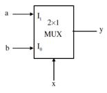
This function can be interpreted as having two inputs a, b and select signal x. Output y will depend on the select signal x. Function will be like (ax+bx') its implementation will be like as shown in fig.
