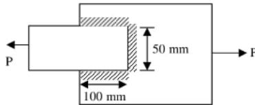
Maximum load taken by plate =  $150 \times 50 \times 8 = 60\text{KN}$
