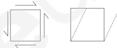
Here since angle has increased, so shear strain should be negative.
