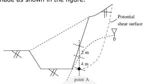
The soil exhibits c'= 20kPa,  $\phi$ =18°, and the undrained shear strength = 80 kPa. The unit weight of water is 9.81kN/m³. The unit weights of the soil above and below the ground water table are 18 and 20 kN/m³, respectively. If the shear stress at Point A is 50 kPa, the factors of safety against the shear failure at this point, considering the undrained and drained conditions, respectively, would be
