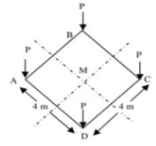
The vertical stress increment (in kPa, up to one decimal place) due to these loads according to the Boussinesg's equation, at a point 5 m right below M, is\_
