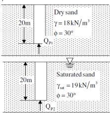
If  $Q_{P1}$  and  $Q_{P2}$  represent the ultimate point bearing resistance of the piles under dry and submerged conditions, respectively, which one of the following statements is correct?
