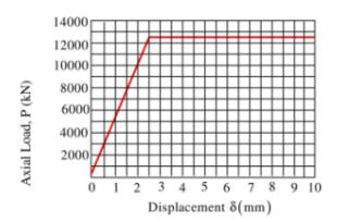
Assume the yield stress of steel as 250 Mpa. The complementary energy (in N-mm) stored in the bar up to its linear elastic behavior will be\_\_\_\_\_
