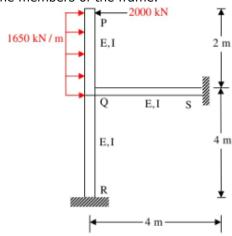
The rotations (in degrees, up to decimal place) at the rigid joint Q would be \_\_\_\_
